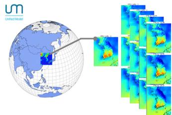
**Figure 2:** LENS specification: The LENS is based on Unified Model (Met Office) which produces 13 ensemble members downscales and forced by global EPS. The grid consists of 460 x 482 x 70 grid points with horizontal spatial resolution 3km x 3km. The LENS provides 72 hours forecast twice a day
