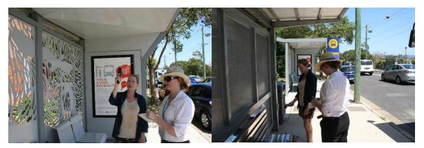
The elements of the design most important to reducing temperature were the provision of additional shade from the larger roof, the insulated roof and placement of seating with respect to shade. Monitoring demonstrated that the CAPS shelter was up to 4°C cooler than the older style bus shelter. Similarly the older style shelter had higher roof temperatures for most of the day, with peak temperatures of up to 15°C higher than the CAPS shelter.
